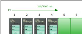
In the SLIO system (Slice I/O), the power consumption of the projected modules is calculated and displayed. Once approximately 70% of the maximum power consumption on the backplane bus has been reached, the colour of the arrow changes from green to orange. Once approximately 90% of the maximum power consumption has been reached, the colour changes to red.
