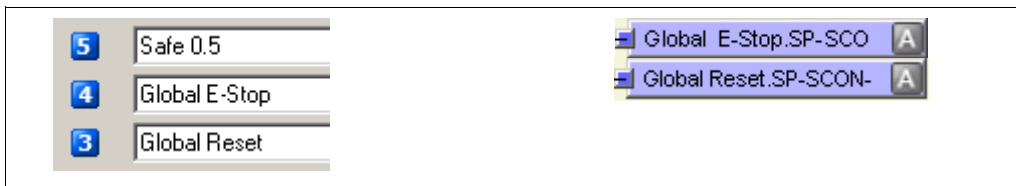
Fig. 53: Assigned samos®NET tag names in the routing configuration and in the logic editor
