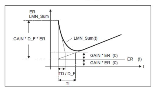
LMN\_Sum(t) manipulated variable in automatic mode of the controller
