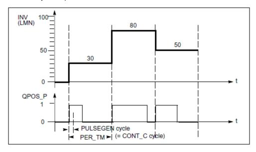
An input variable of 30% and 10 FB PULSEGEN calls per PER TM means the following:
