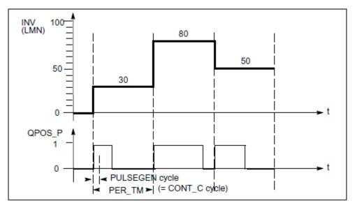
An input variable of 30% and 10 FB PULSEGEN calls per PER\_TM means the following:
