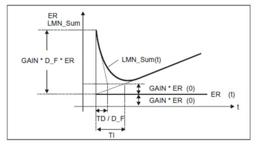
LMN\_Sum(t)manipulated variable in automatic mode of the controllerER (0)step change of the normalized errorGAINcontroller gainTIintegral timeTDderivative timeD\_Fderivative factor
