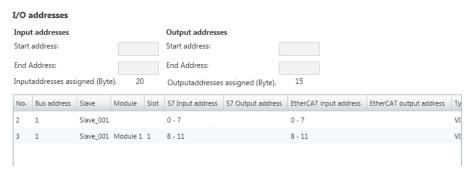
Here you have a list of S7 respectively EtherCAT addresses, which are used by the modules of the slave system. The 'S7 address' corresponds to the address in the address area of the CPU. By entering a new 'Start address' you can adjust the S7 addressing of the input and output areas of the modules accordingly.
