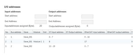
Here you have a list of S7 respectively EtherCAT addresses, which are used by the modules of all the slave stations. The 'S7 address' corresponds to the address in the address area of the CPU. By entering a new 'Start Address' you can adjust the S7 addressing of the input and output areas of the modules accordingly.
