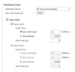
This dialog is only visible in the 'Expert mode' if this is supported by your slave station! Here you can adjust the clock functionality accordingly. In EtherCAT "Distributed Clocks" (DC) means a logical combination of "clocks", which are located in the EtherCAT devices. With this there is the possibility to locally provide a synchronized time in each bus device. If an EtherCAT device supports the Dis-
