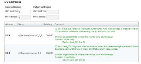
Here you have a list of addresses, which are used by the I/O components of the modules of the selected slave system in the address area of the CPU. By entering a new 'Start address' you can adjust the addressing of the input and output areas accordingly. You can edit 'Name' and 'Comment' by clicking at the corresponding entry.
