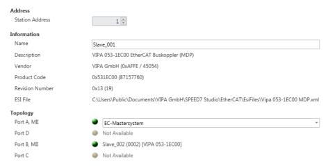
Here you can perform slave-specific settings such as assignment of name and address to a station. It is also possible to change the connection to the station.
