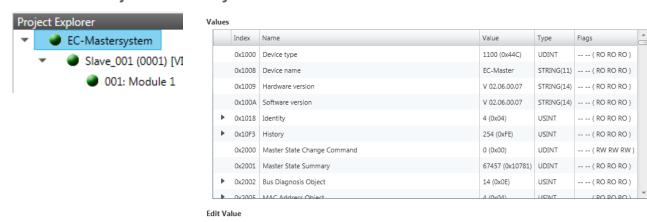
Here you will have read and write access to the CoE Object Dictionary of the slave station. This can be changed if your slave station permits. It is indicated by the *'Flags'* of each object, if write access is permitted. Information about the structure of the Object Dictionary can be found in the manual of your slave station.
