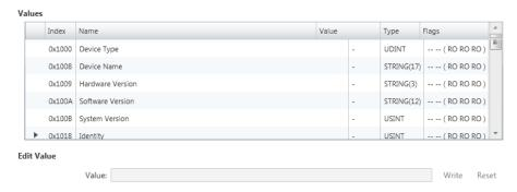
This dialog is only visible in the 'Expert mode'! Here you will have read and write access to the CoE Object Dictionary of the slave station. This can be changed if your slave station permits. It is indicated by the 'Flags' of each object, if write access is permitted. Information about the structure of the Object Dictionary can be found in the manual of your slave station.
