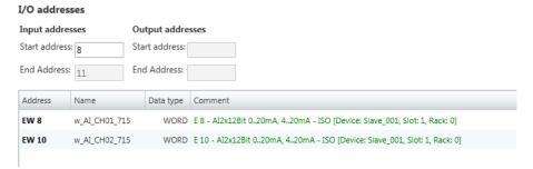
Here you have a list of addresses that are used by the module in the address area of the CPU. By entering a new 'Start address' you can adjust the addressing of the input and output areas accordingly. You can edit 'Name' and 'Comment' by clicking at the corresponding entry.
