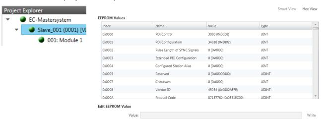
This dialog is only visible in the 'Expert mode'! Here you can access the contents of the EEPROM of the slave station. Currently you can only change the parameter 'Configured Station Alias'. This can be used for forming groups. § Chapter 3.10 'Grouping logic' on page 45
