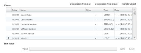
Here you will have read and write access to the CoE Object Dictionary of the slave station. This can be changed if your slave station permits. It is indicated by the *'Flags'* of each object, if write access is permitted. Information about the structure of the Object Dictionary can be found in the manual of your slave station.
