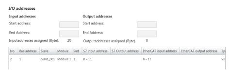
Here you have a list of S7 respectively EtherCAT addresses, which are used by the modules of all the slave stations. The 'S7 address' corresponds to the address in the address area of the CPU. By entering a new 'Start Address' you can adjust the S7 addressing of the input and output areas of the modules accordingly.
