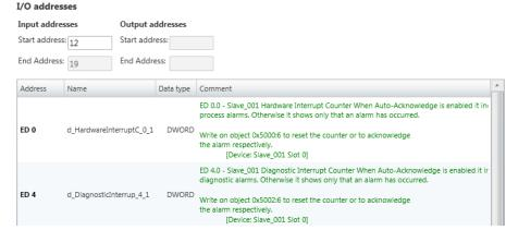
Here you have a list of addresses that are used by the I/O components of all the modules in the address area of the CPU. By entering a new 'Start address' you can adjust the addressing of the input and output areas accordingly. You can edit 'Name' and 'Comment' by clicking at the corresponding entry.
