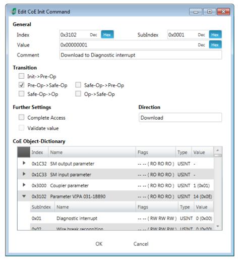
**This dialog is only visible in the 'Expert mode'!** With [New] the dialog 'Add CoE Init Command' opens. This dialog also opens to edit CoE Init Commands, which just exist.
