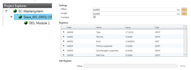
This dialog is only visible in the 'Expert mode'! Here you can directly access the registers of the EtherCAT ASIC. You should not make any changes here!
