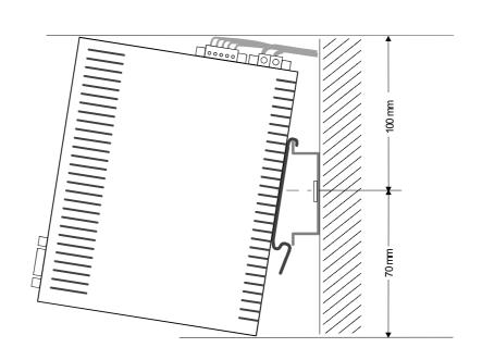
Insert the module that you are installing into the profile rail at an angle
