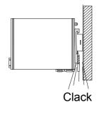
• Insert the module that you are installing into the profile rail at an angle of about 45 degrees from the top and rotate the module into place until it clicks into the profile rail with an audible click.
