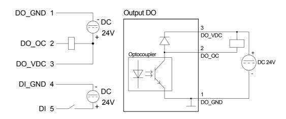
DI/DO wiring / schematic diagram
