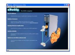
• Switch to the list view with "Switch to list mode". Here every TM-E module available in you network is listed.
