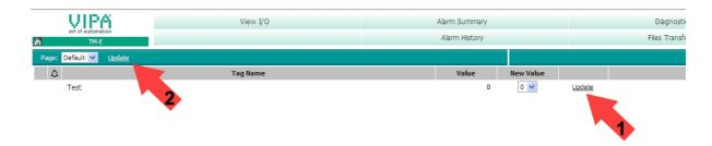
• If the new value is accepted by the CPU, so the communication between the TM-E module and the CPU is secured.
