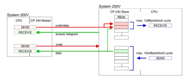
Access to multiple At deployment of multiple slaves with RS485 there cannot occur bus conflict errors because the master may only communicate with one slave at a time. The master sends a command telegram to the save specified via the address and waits for a certain time where within the slave may send its respond telegram. During the latency communication with another slave is not possible.
