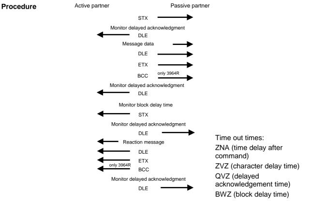
Timeout timesThe QVZ is monitored between STX and DLE and between BCC and DLE.ZVZ is monitored for the entire period of receiving the message.
