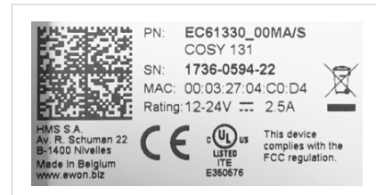
Fig. 4 Ewon Cosy 131 — 4 ports Ethernet: Label
